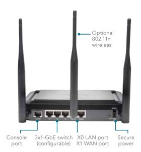
address the demands of deep packet inspection at high traffic loads. The SonicWall TZ Series platform relies on processors that, unlike x86, are optimized for packet, crypto and network processing while retaining flexibility and programmability in the field — a weak point for ASICs systems. This flexibility is essential when new code and behavior updates are necessary to protect against new attacks that require updated and more sophisticated detection techniques.
